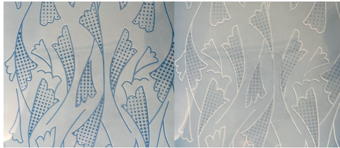
An electrochromic display is a dynamic free-form shape-based display. The shape and patterns are defined at the time of their creation.
