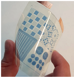
An electrochromic display is flexible.
