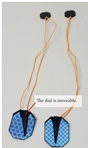
The pendant showing a different pattern triggered by the movement of remote dial. The chain could be removed and be worn as a pin.
