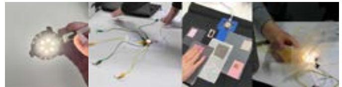
Figure 1. From the left: 1) The Light Up Board is quite small. 2) Participant P3 testing the touch sensors on the Light Up Board using copper tapes. 3) Participant P6 testing her prototype after integrating the Light Up Board with her custom-made touch sensors and other components. 4) Participant P1 testing material to create a flame-like feeling from the Light Up Board.
