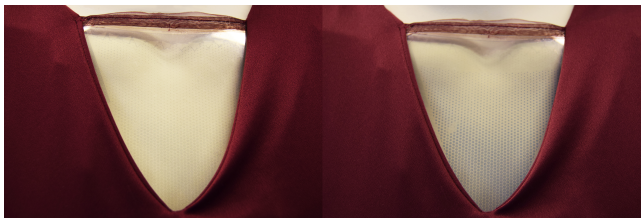
Figure 7: Left: The display in transparent state, revealing the low neckline. Right: Display opaque mode, covering the neckline.
